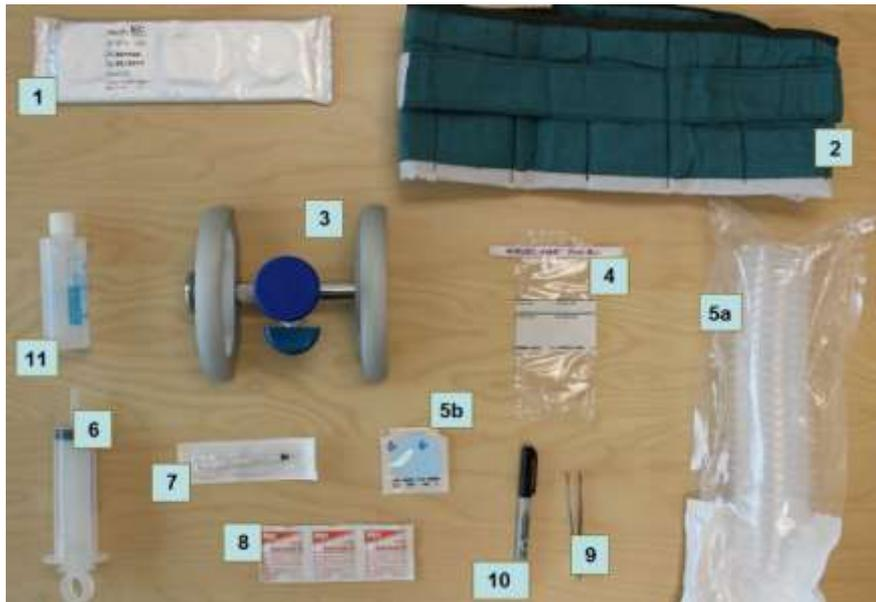
**Figure 1: Equipment required for water quality testing**
